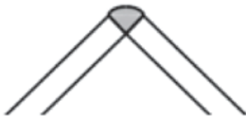
Corner Weld (Fig 1-19g)
